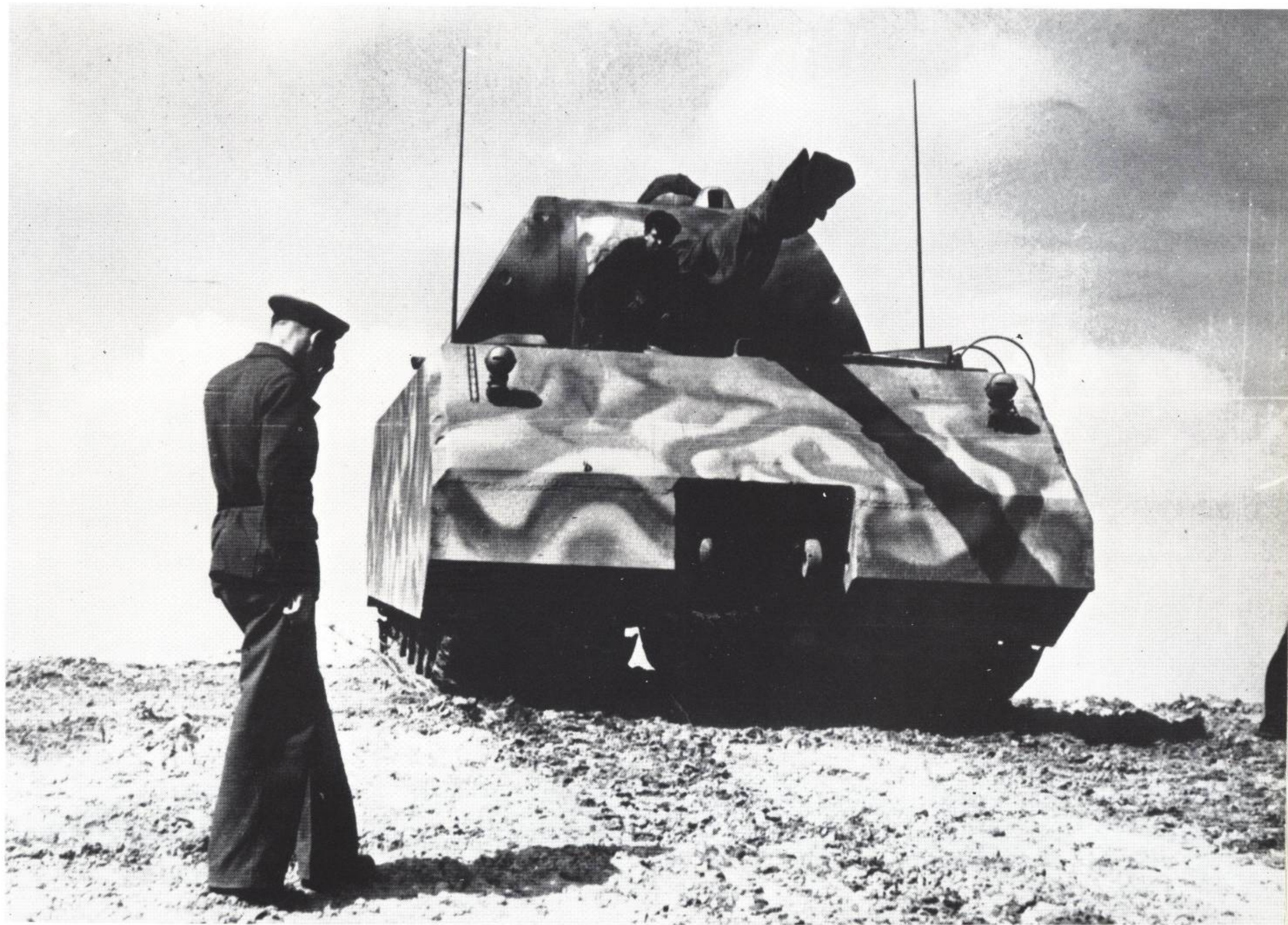
An imposing front view of the Maus, showing the two antenna staffs. Aiming the cannon was done with the help of an elevation gauge, aiming telescope and elevating machine operated by the gunner. The arc of elevation ranged from -7 to +23 degrees.
