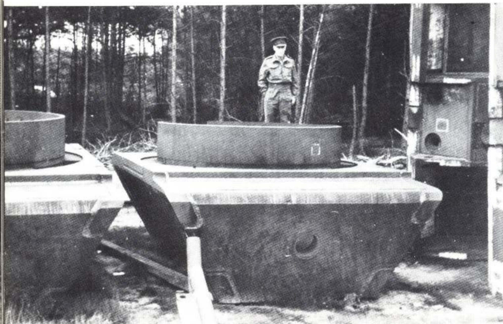
Above: Along with the two completed Maus tanks, there were three others under construction. Parts of them were found by the Allies at the Krupp factory in Essen. Here are two turrets; at the right edge of the picture a hull standing on end is recognizable. Below: View through the gun aperture into the interior of a turret casting. The ammunition hole is in the rear wall. 24 of the total of 68 shells for the 12.8 cm cannon were to be stored against the rear wall, while 125 of the 200 7.5 cm shells were intended to be stored in the turret.
